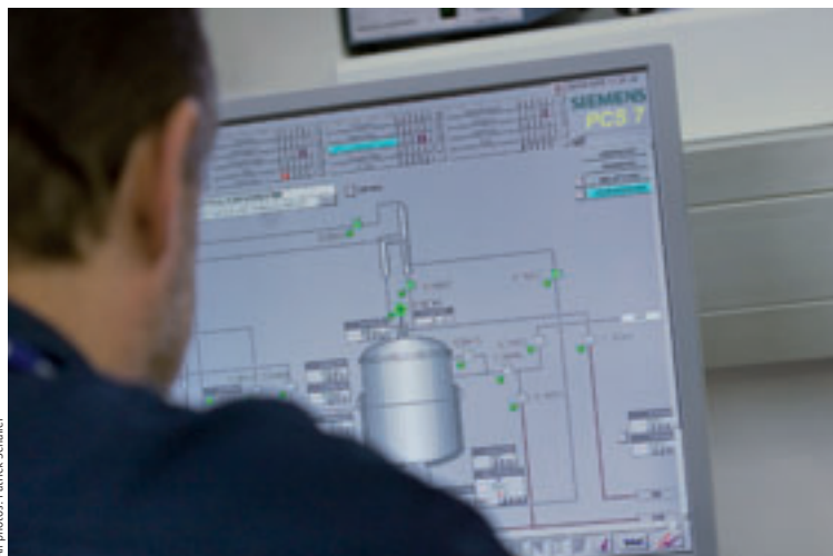
Simatic PCS 7 and Simatic Batch: the process control system and batch software ensure fully automatic recipes in research and production
