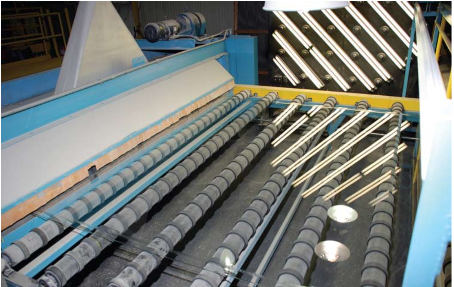
Glass is tested for proper thickness across its entire width. Any defects are discarded and recycled.
