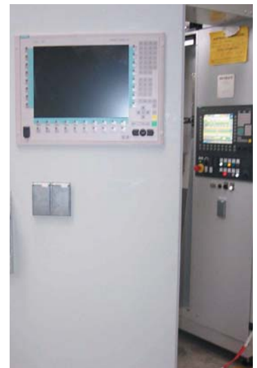
Left and Above: Cell controller used for monitoring and control of all machines within the cell
