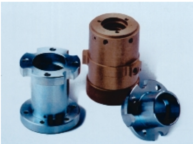
Typical parts machined and fabricated by Zephyr include these hubs for amusement park equipment.
